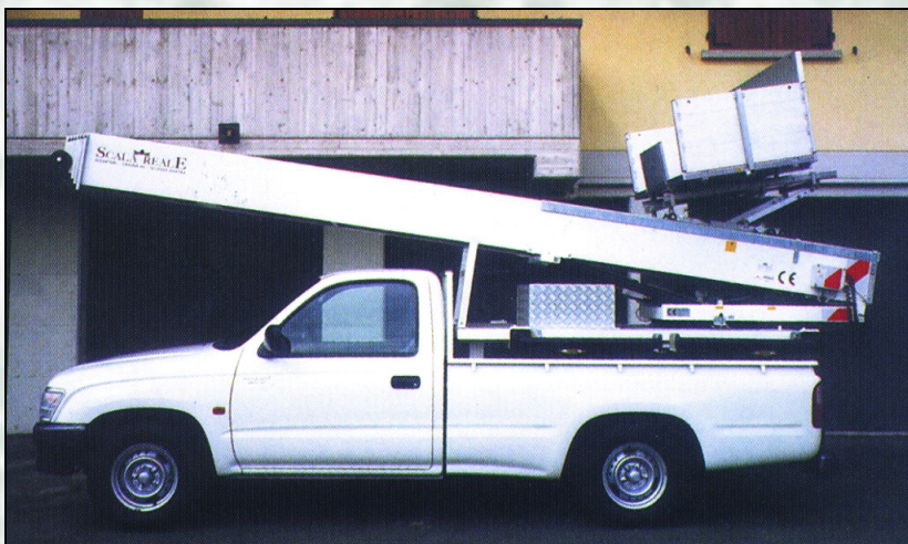
In the extractable version, the ladder is fitted in the back and may be separated at convenience. In this case the lift is considered as outrigger load. Alternatively, the ladder truck comes as a fixed unit approved for travel on road as a special transportation vehicle.
