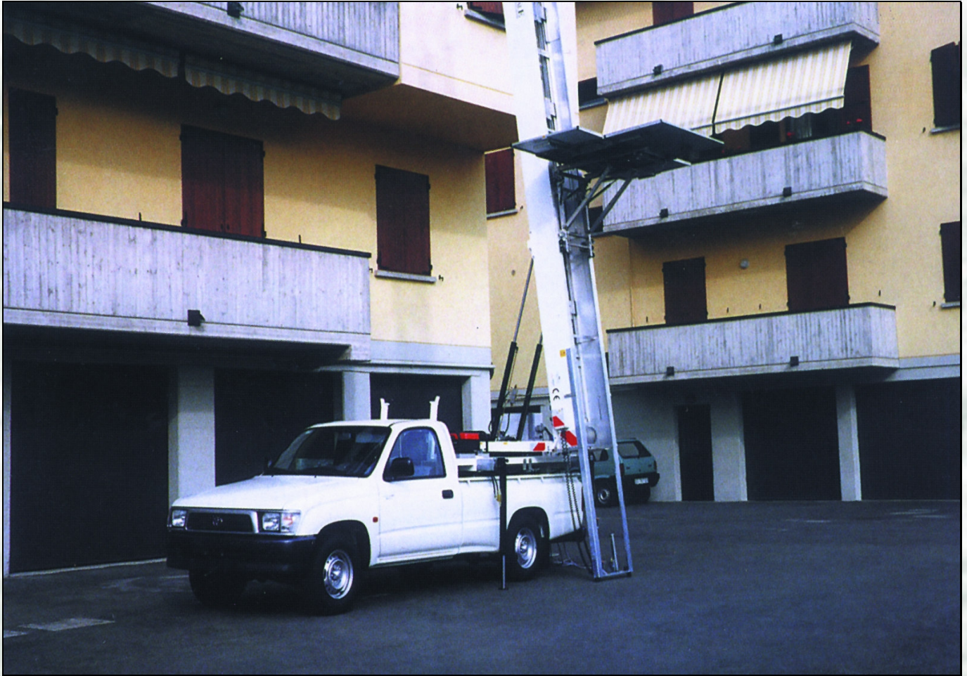
The above picture shows a typical version of the pick-up model Dedalo 7.5050 (30.5 m high) mounted on TOYOTA HI-LUX 2WD ladder truck with 4 hydraulic stabilizers (standard) and gasoline engine (optional) with aluminium casing.
