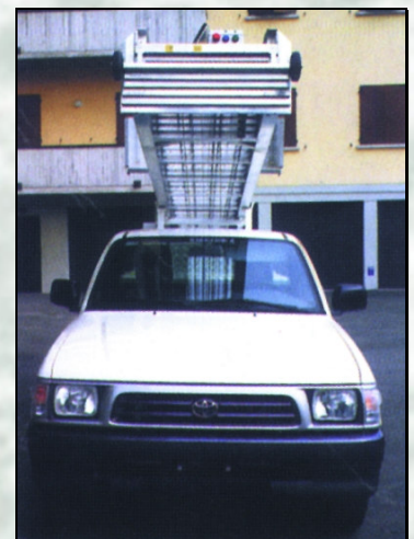
The maximum ladder height on TOYOTA HI-LUX 4x2 is approximately 2.4 m.
