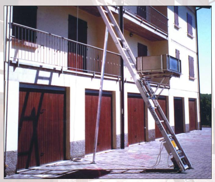
Whenever sufficient space is available on site, the lift may be flat mounted on ground and raised up after mounting. Alternatively it is possible to perform vertical mounting by means of the optional electric hoist and ropes.
