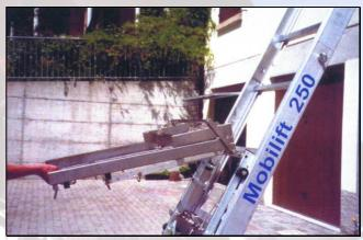
The loading platform support is made out of stainless steel and is quickly and easily coupled to the platform by means of 2 locking pins. Leveling of the platform is accurately performed by means of telescopic channels.
