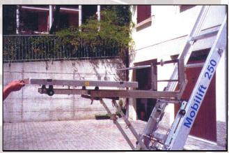
The work platform is turning and fitting into window dimensions. Sliding is performed by means of special guides on the support. All 3 loading platform extensions are removable and suitable for either horizontal or vertical setting.
