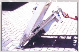
The electric motor is equipped with own wheels so that no lifting is required for mounting operations. Fixation of the electric motor to the base is assured by one single locking pin. The frame, the motor and the reduction gear are made out of aluminum.
