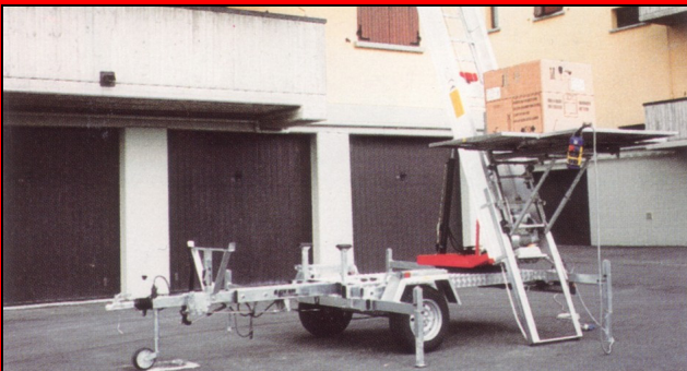
Once the lift is in place the drawbar can be pulled back to fit into a smaller parking place.
