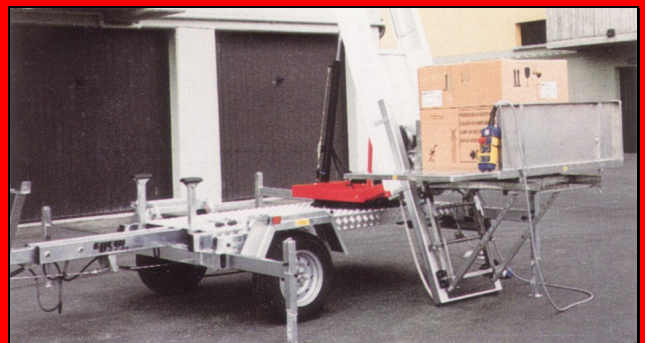
The loading platform may be rotated to fit into the windows or balcony size. A platform extension makes loading and unloading easier.
