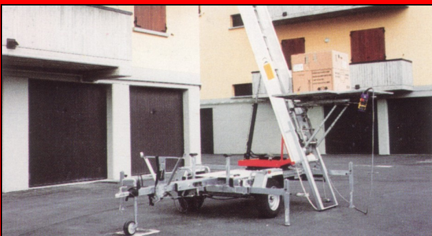
All telescopic sliding sections are made out of aluminum EN AW-7020 assuring 200 kg rated load. All operations are performed electrically and controlled on a push-button panel; on the top of the lift a push button for down and stop operations is available.
