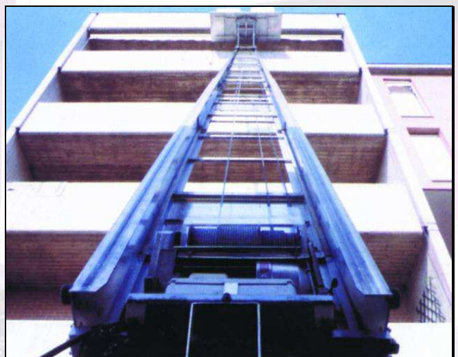
Load capacity: 200 kg at the maximum height
