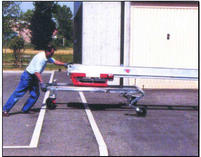
Going up a step by unbalancing the lift
