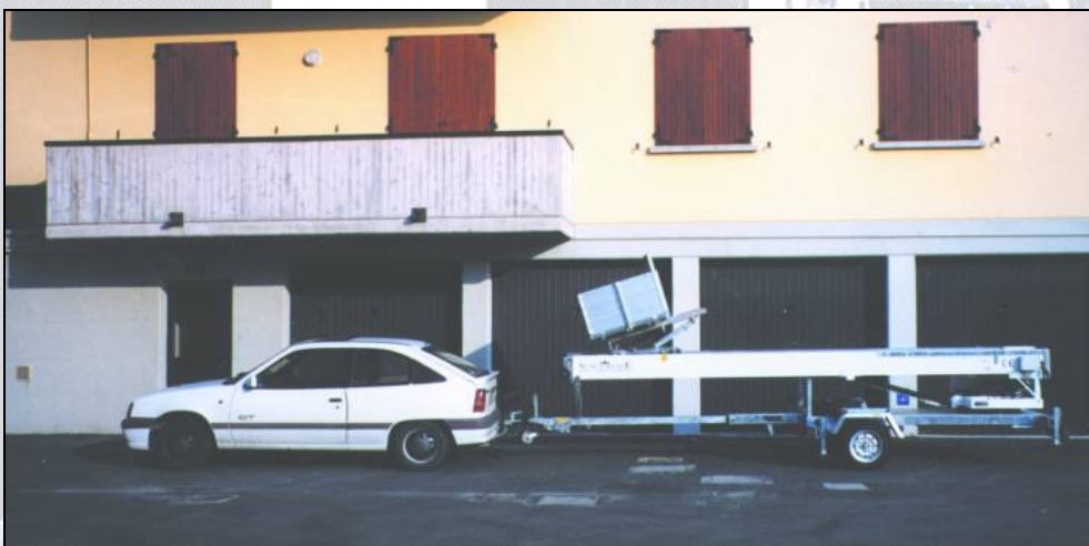
The trailer is equipped with parking brakes and inertial brakes in compliance with European Directives no. EC/91/422. Because of reduced weight (750 kg - 1000 kg depending on the model) towing is possible with most commercial cars and vehicles. Installation on a 750 kg total mass trailer is possible up to 23 m height.
