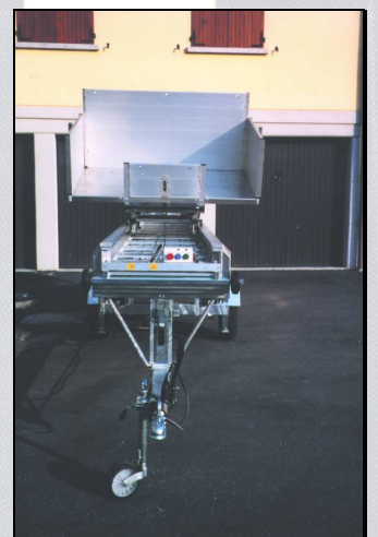
Up and down as well as safety stop buttons are available on the lift top. The platform front panel is both foldable and removable.
